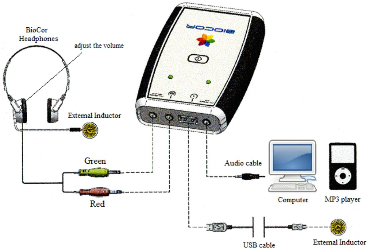
Fig.2. BioCor connections
