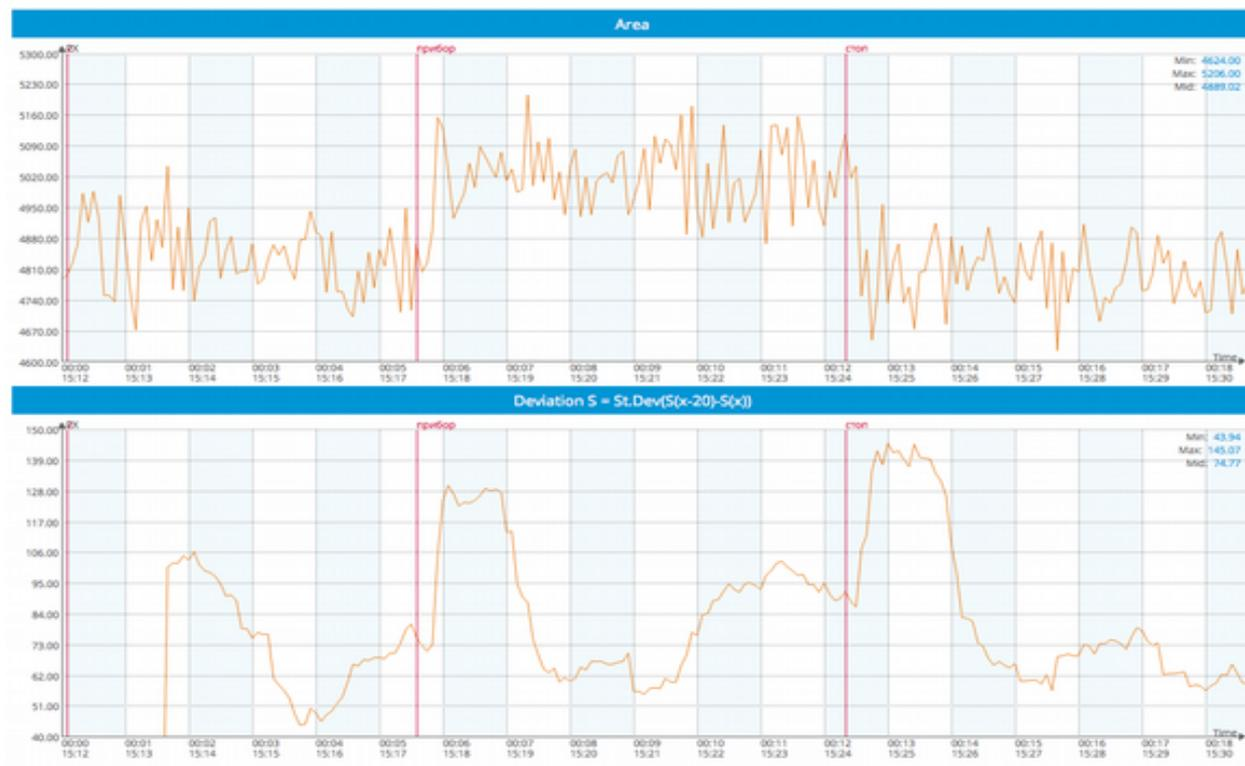
*Example 1: Response of water to high frequency electromagnetic fields (generator is turned on and off).*
