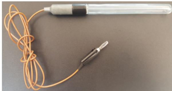
*Pic. 1. Water sensor for the Bio-Well device.*
