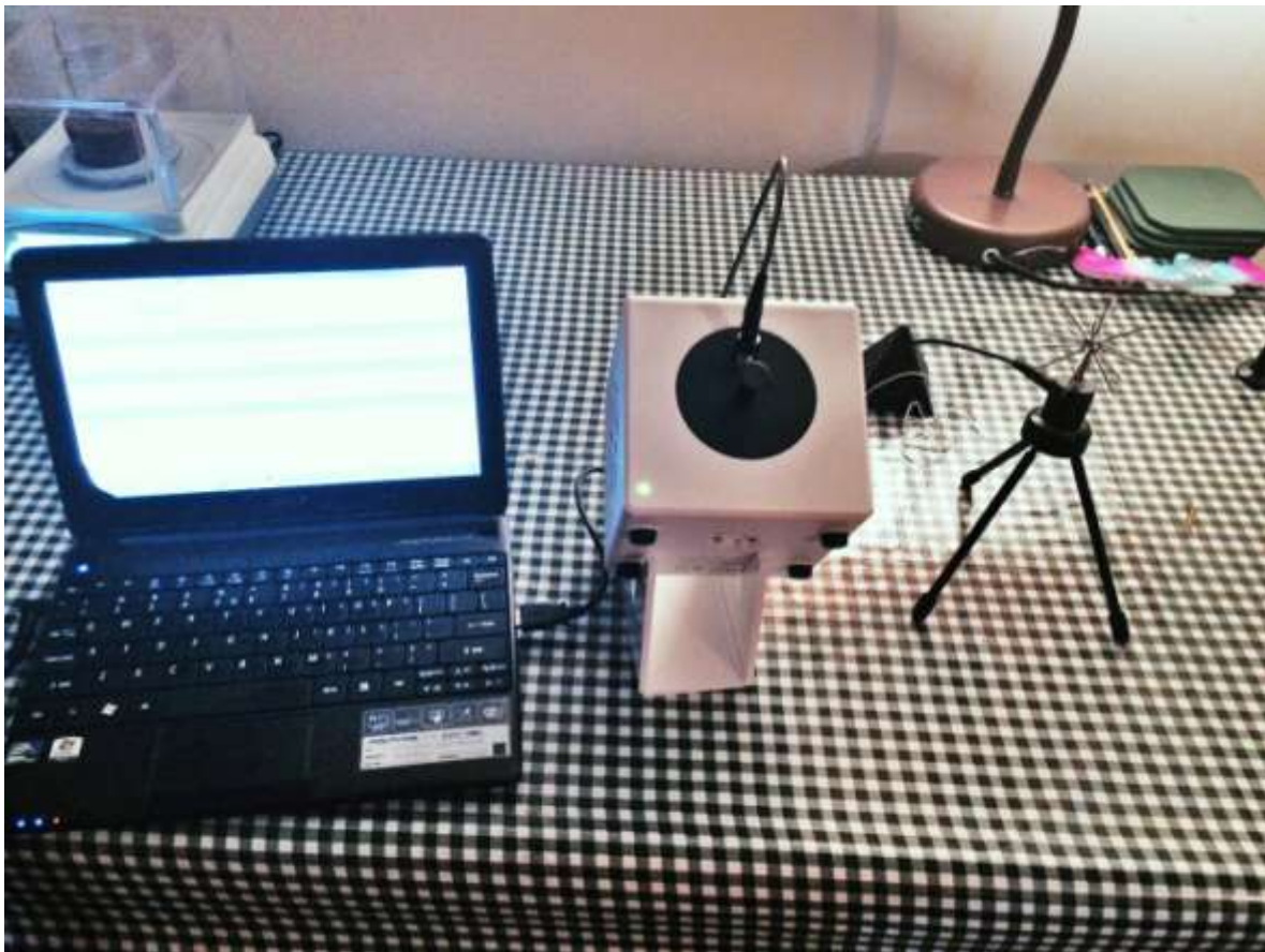
Figure 1. Photograph of experimental setup, showing the Bio-Well instrument (center) positioned on its stand, with the metal cylinder (calibration unit, not visible here) inserted into the front (black circular region), to which Sputnik sensor (right) is connected by a wire lead.
